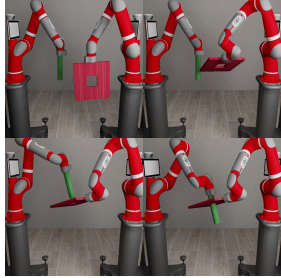
Two Arm Peg-In-Hole: Two robot arms are placed either next to each other or opposite each other. One robot arm holds a board with a square hole in the center, and the other robot arm holds a long peg. The two robot arms must coordinate to insert the peg into the hole. The initial arm configurations are randomized at the beginning of each episode.
